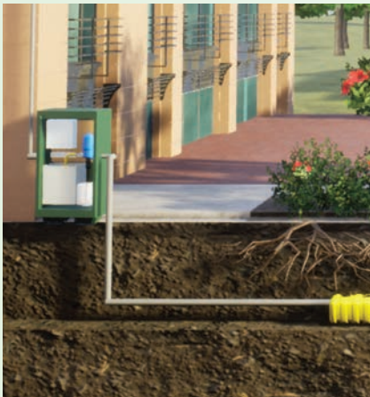
Pump communicates with water level sensor and activates when water tank level is low
